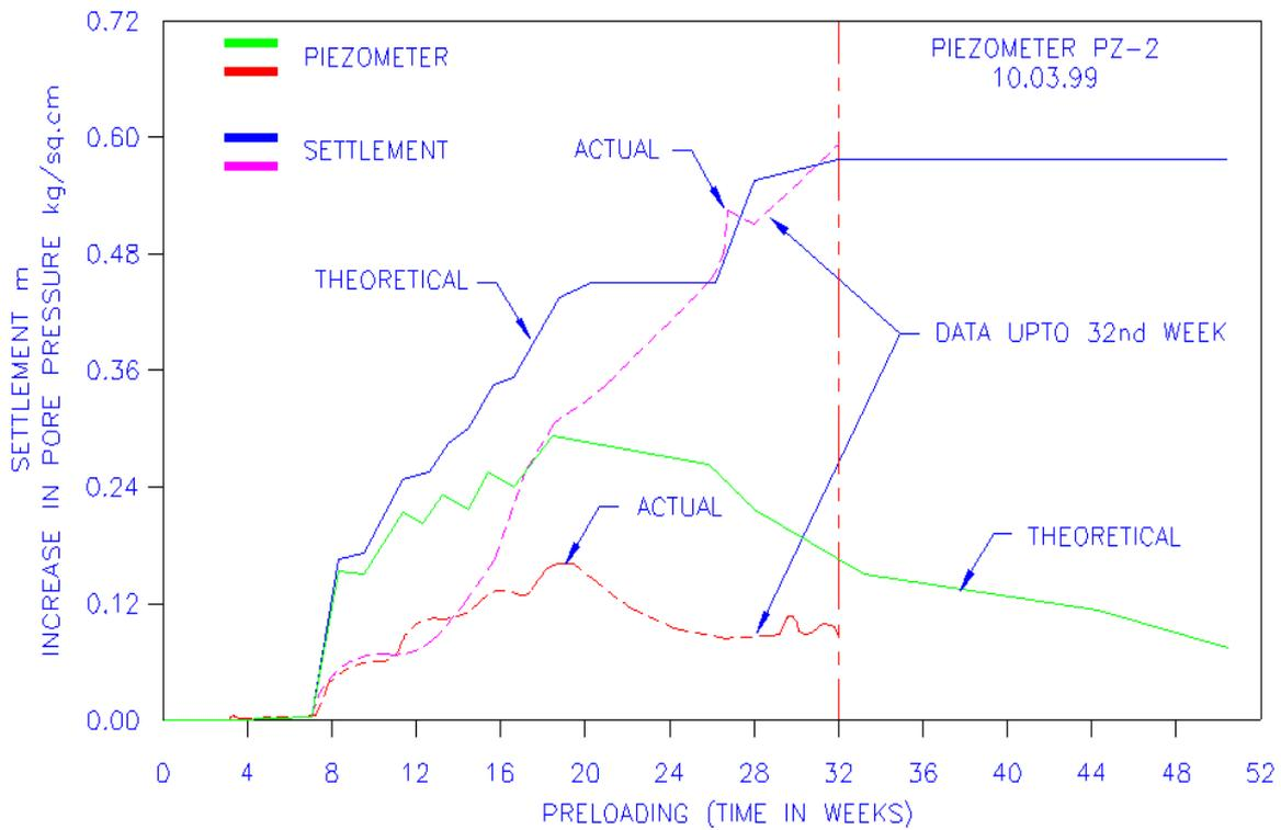
FIGURE 3.2: READINGS OF PIEZOMETER PZ-2 FOLLOWING EXPECTED TREND
