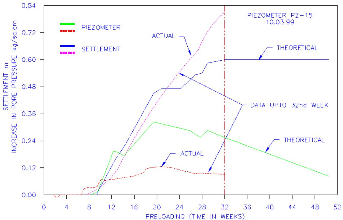
FIGURE 3.3: READINGS OF PIEZOMETER PZ-15 SHOWING CONSTANT OUTPUT
